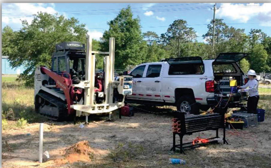
EGS Performing CPT / HPT / Conductivity Logs and Setting Cased Hole Piezometers for Infiltration Properties
