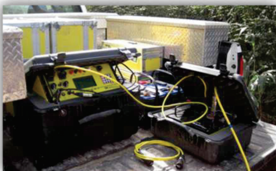
ERI Data Collection & Control Units
