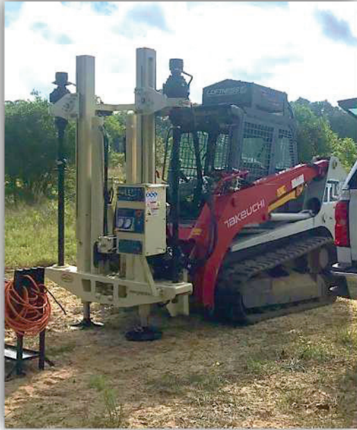
EGS performing CPT / HPT / Conductivity Log
