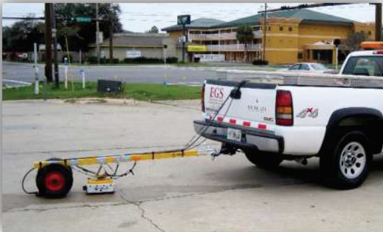
800 MHz GPR Antenna on Road Trailer
